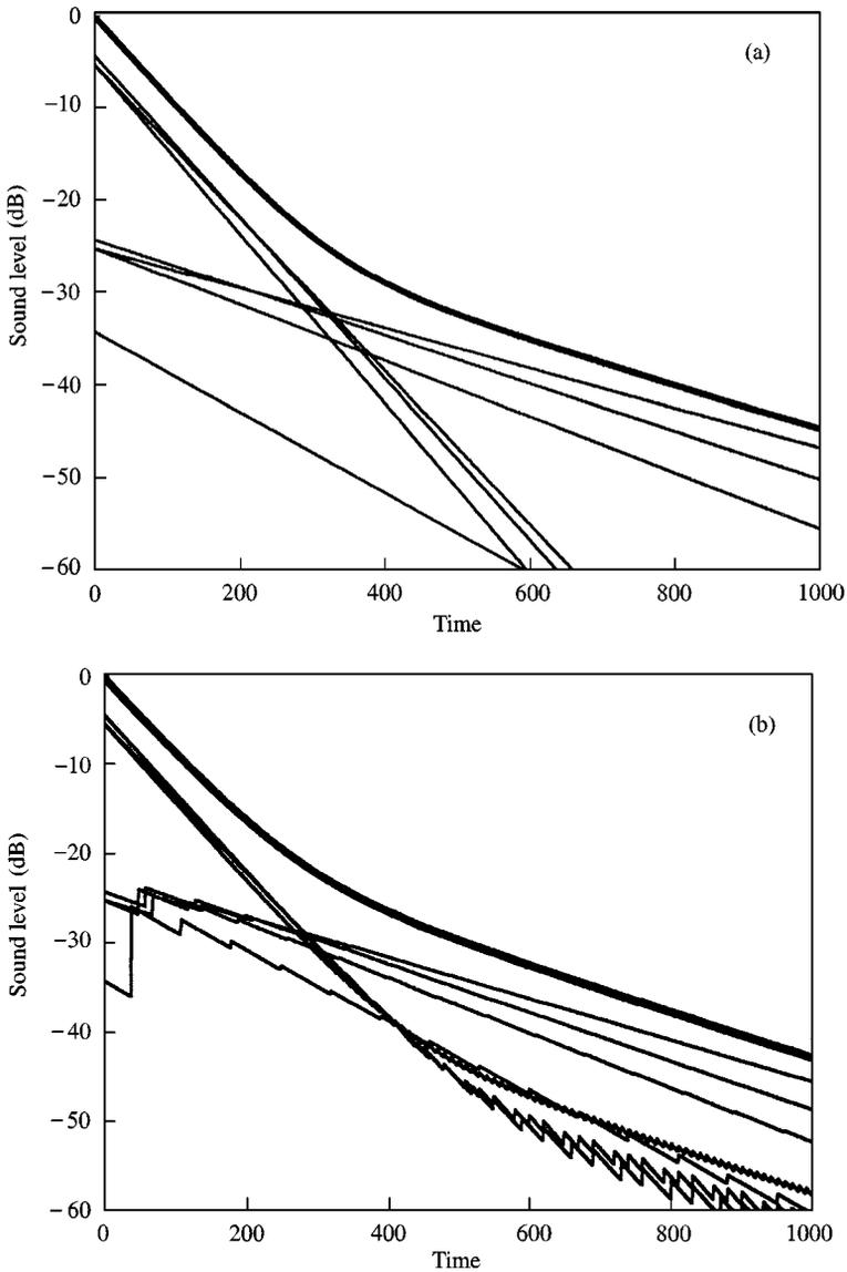
Figure 6. Energy decay curves of a coupled room. Examples of individual curves of free path categories and total decay curve (—). (a) Without transition between the categories; (b) with transition between the categories.
