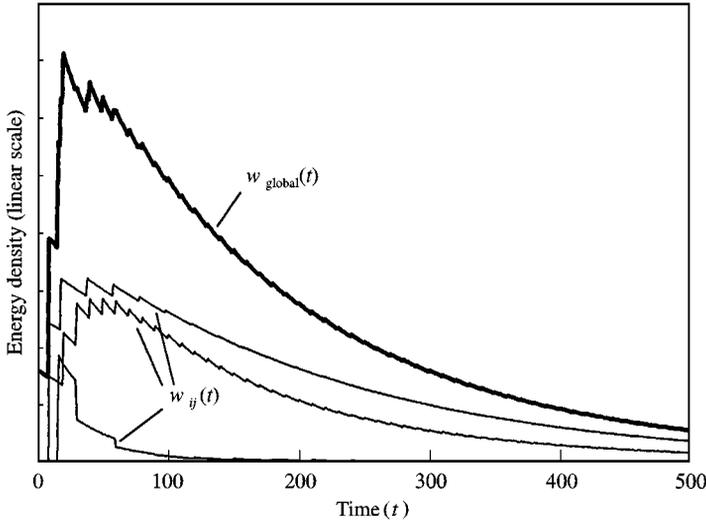
Figure 3. Individual and global decay processes with transition between free path and absorption categories.
