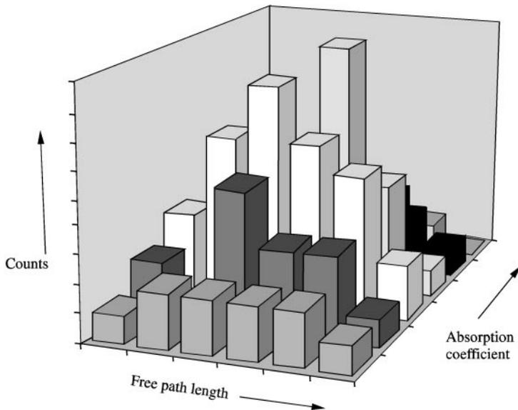
Figure 2. Matrix of statistical distribution of free path lengths and absorption coefficients.
