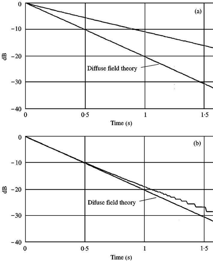
Figure 4. Sound propagation curves in a flat room ( $100 \times 100 \times 4 \text{ m}^3$ ): (a) specular; (b) diffuse reflections.
