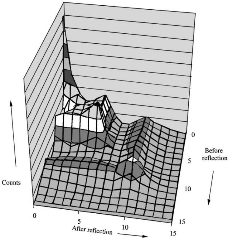
Figure 5. Free path distribution matrix of coupled rooms with uniform absorption.
