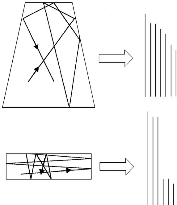
Figure 1. Relation between room shape and free paths, top: “normally” shaped room, bottom: flat room. The lengths of free paths are recorded and put into an order according to their length.
